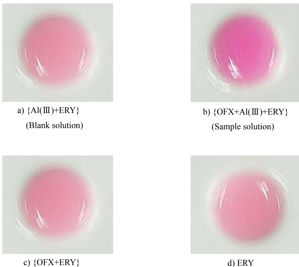
Fig. 2-4 Color reaction on white spot plate a)Al(III)-ERY solution; b)OFX-Al(III)-ERY solution; c)OFX-ERY solution; d)ERY solution.
