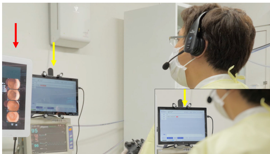
Fig. 2 Endoscopic reporting system with voice recognition technology during the procedure. This image shows the voice recognition system used for report preparation during the procedure. An endoscopist wearing a headphone with a microphone is pronouncing the endoscopic finding while looking at an endoscopic picture on a
